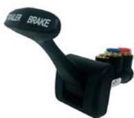
Trailer Brake Valve C/V 3 Freightliner 265031
