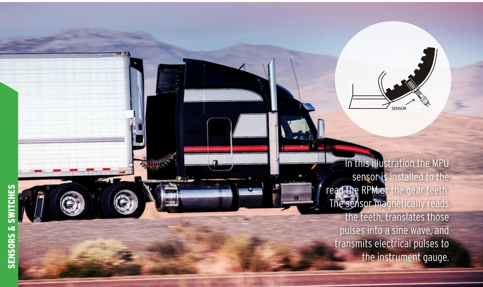
In this illustration the MPU sensor is installed to read the RPM or the gear teeth. The sensor magnetically reads the teeth, translates those pulses into a sine wave, and transmits electrical pulses to the instrument gauge.
