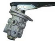
E-6 Foot Brake Valve With Pedal
